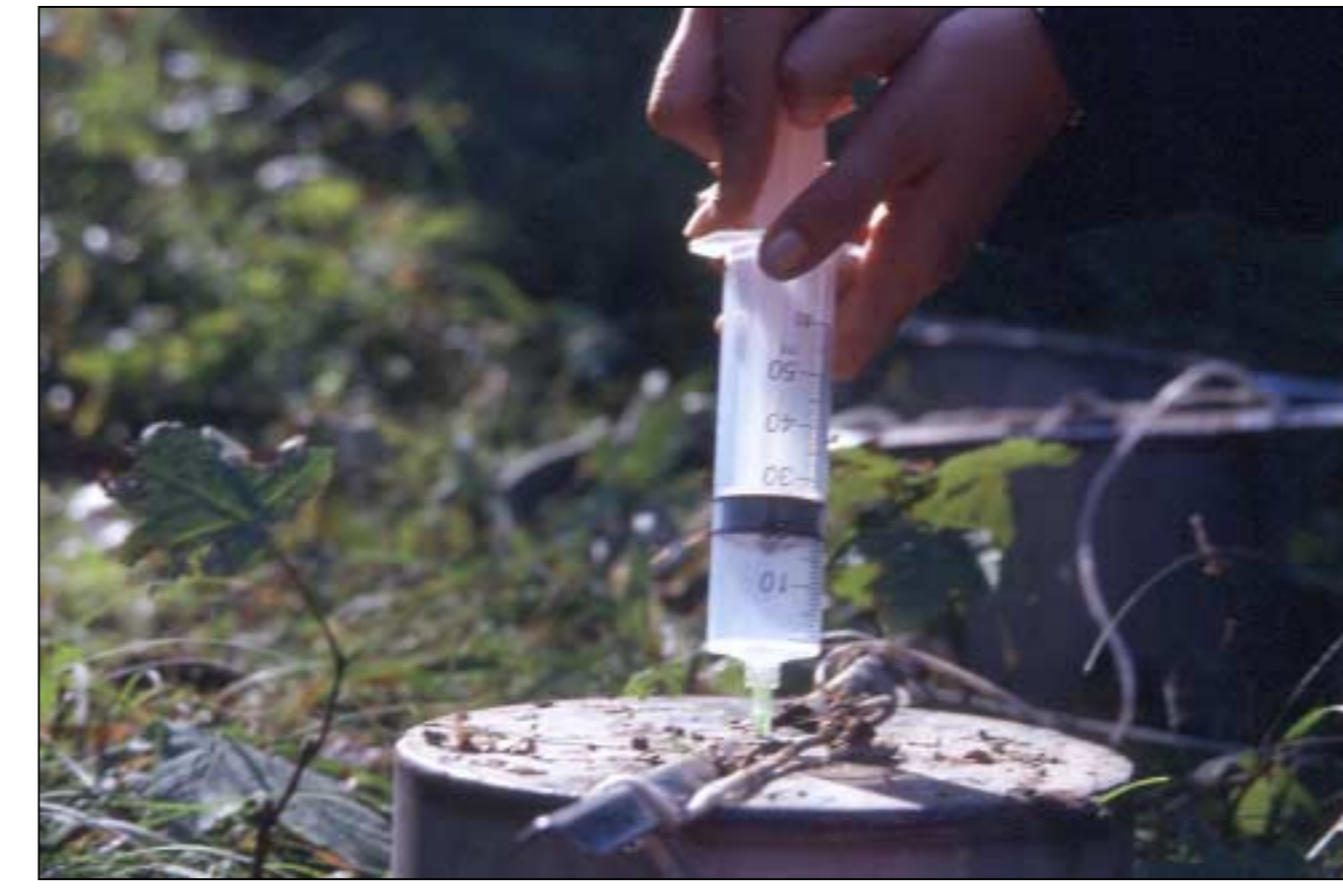
Figure 3. Gas samples taken from static chambers used for the determination of greenhouse gas emissions.
